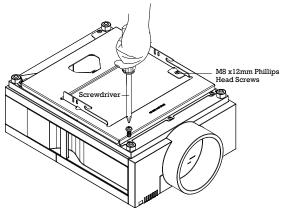
**Step 1**. Using a screwdriver, secure the mounting bracket using eight (8) M8 x 12mm Phillips Head screws.
